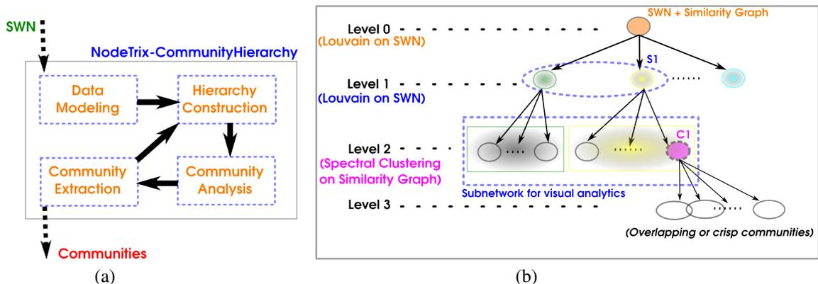
Fig. 1. (a) Our proposed set of techniques, NodeTrix-CommunityHierarchy, for visual analytics of SWNs. (b) Schematic diagram of four-level community hierarchy in a SWN, constructed by using its metadata to generate the similarity graph and choosing nodes and community detection algorithms for further division.
