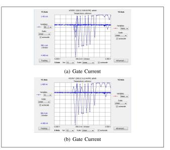
Figure 2: Noise in Gate Current
