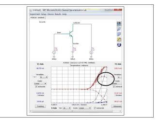
Figure 1: Rise and fall of collector current
