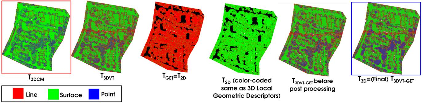
Fig. 1. In Area-2 of Vaihingen dataset (266,675 points),  $T_{3D}$  improves line- and point-type feature detection, thus, distinguishing gabled roofs and foliage, respectively.  $T_{3DVT}$  detects (77,679, 173,991, 15,005) points as (line, surface, point)-type features;  $T_{3DVT-GET}$  detects (73,332, 68,175, 25,168), and  $T_{3D}$  detects (64,849, 158,937, 43,889), respectively.
