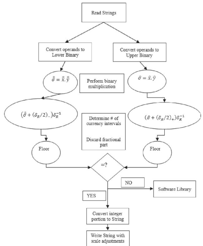
Fig. 13. Flow chart for performing multiplication transactions (database to database cycle).
