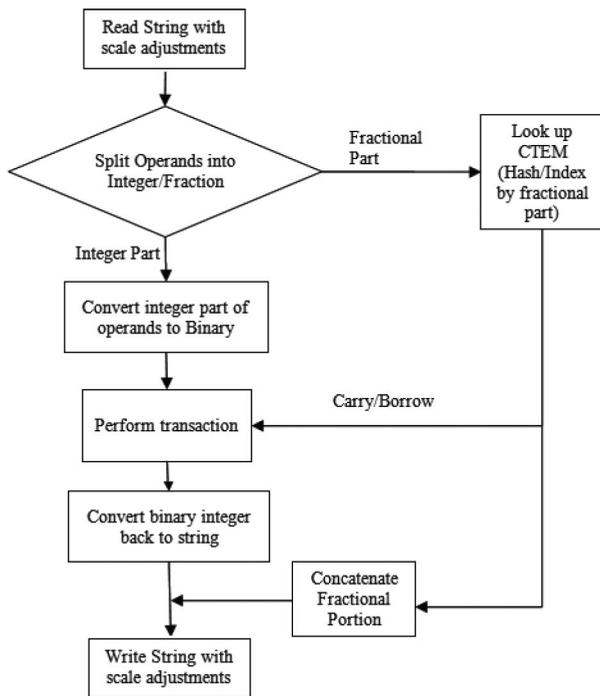
Fig. 11. Flow chart for performing addition/subtraction transactions (database to database cycle).
