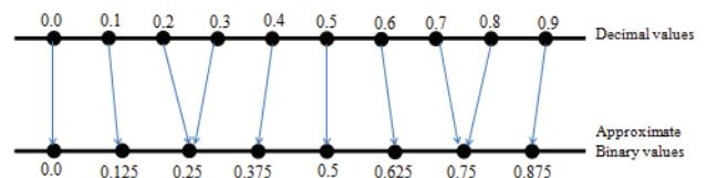
Fig. 5. Mapping decimal values (with one place of significance) to the corresponding approximate binary values (of three significant bits).
